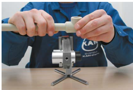
Fig. 3.15. Immobilising the pipe with the elbow fitting in the PP system
