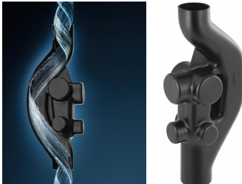
Fig. 3.88 Among many accessories, such as drains, cleanouts, horizontal branches and system fittings, Geberit offers also a unique monolithic fitting system for connection of sewage system levels from the sanitary facilities, called Geberit Sovent. This element ensures high time savings in installation of raisers and increases the admissible capacity of raisers in relation to the solution based on traditional couplers with the same diameter
