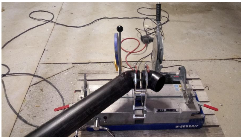
Fig. 3.84. Welding machine for butt welding, equipped with a mechanical plane and heating plate. (own source)
