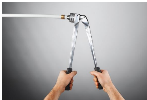
Fig. 3.41. Swelling a pipe with a tool dedicated to TECEflex
