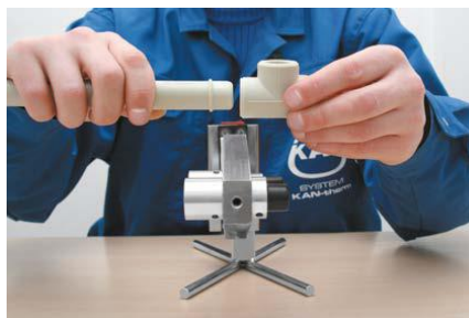
Fig. 3.14. Joining the pipe with the elbow fitting in the PP system
