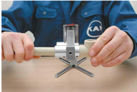
Fig. 3.13. Welding the pipe with the elbow fitting in the PP system
